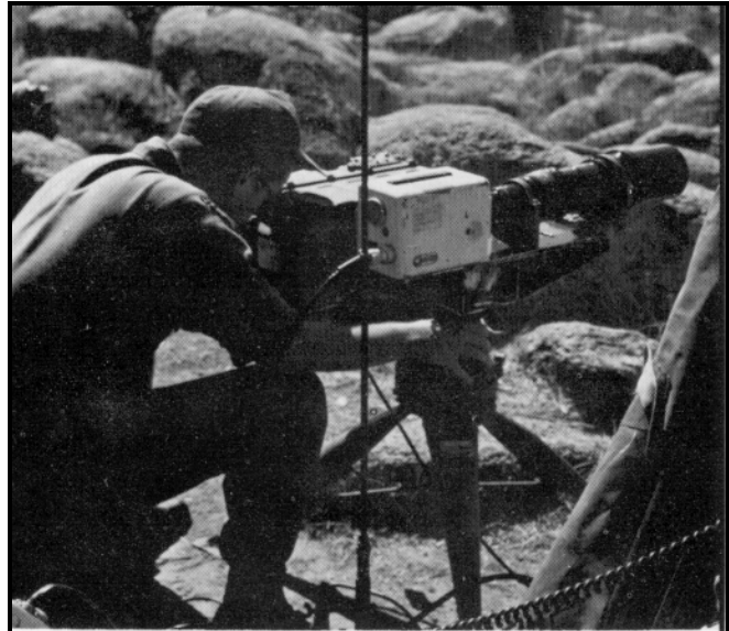
FO lases target using ground/vehicular laser locator designator. Camera mounted on G/VLLD nightsight records data for simulated cannon-launched guided projectile.
