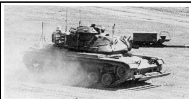
Moving across open terrain, an M60 tank approaches a minefield during a simulated attack on an opposing force. The unusual bumperlike device at the front picks up signals from simulated mines. The large box on the main guns contain electronic instrumentation for relaying those signals between the tanks and CDEC's computerized data-gathering device.
