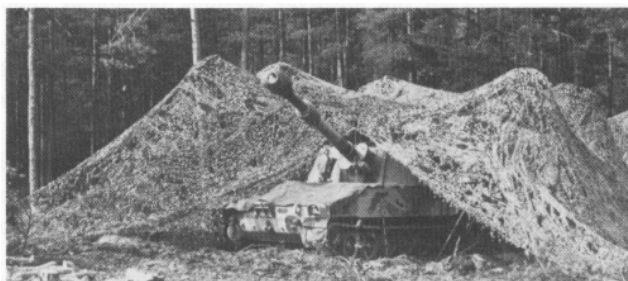
A howitzer section from the 1-3d FA, 2d Armored Division, awaits a fire order deep in German woods after its "deliberate occupation" part of the section ARTEP. In this portion of the test, a section has 30 minutes to set up, camouflage, establish security and prepare to fire.
