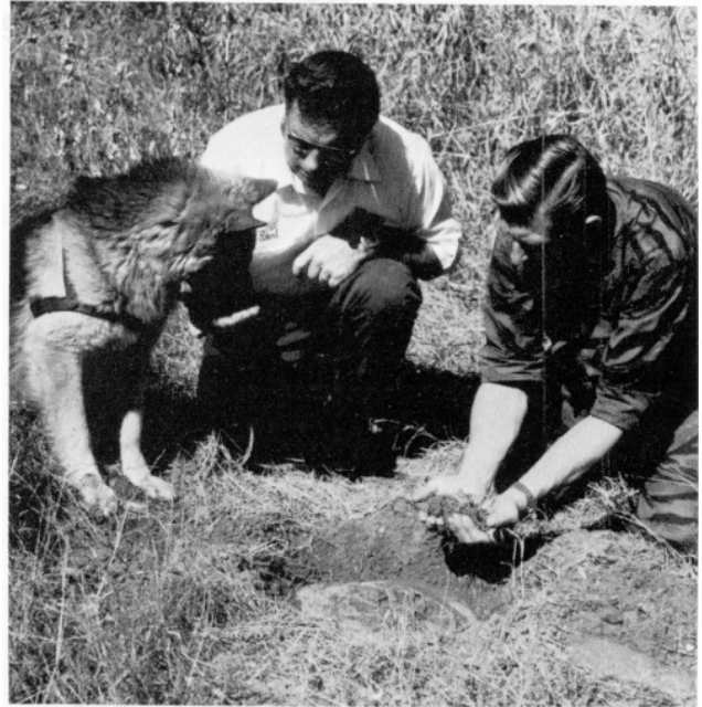
Baron, a German shepherd, locates antipersonnel mines by detecting the odor emitted from the explosive. Dogs have located explosive devices before but only by sniffing out the human scent associated with their emplacement.
