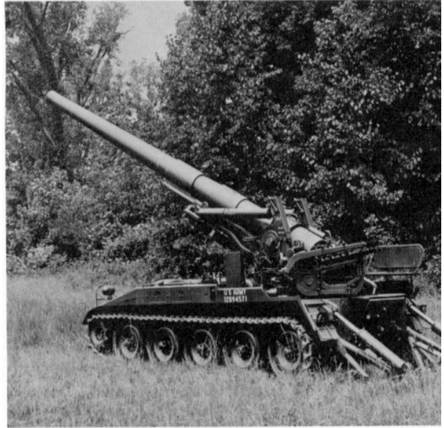
Now classified as a standard item in the field artillery inventory, the M110A1 8-inch howitzer will replace the M110 and M107 by 1979.
