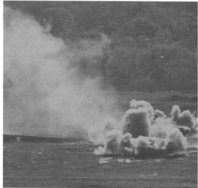
Exploding on impact, 40-mm rounds were included in the recent CDEC suppression experiments. Field exercises evaluated the effects of 15 weapons ranging in size from the infantry rifle to the 8-inch howitzer.
