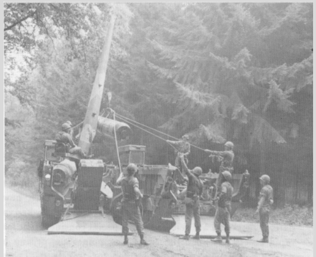
Figure 5 — Rapid Transload of Second Missile. As soon as the first missile is fired the loader transporter is moved to an open area and configured for a rapid transload while the launcher is enroute. A second missile is quickly loaded onto the launcher.
