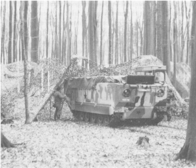
Figure 2 — Camouflage for Lance. Nets are erected on a priority basis immediately upon occupying a position. All vehicles are covered by nets and all missile-handling operations involving exposure of missiles or missile containers are accomplished under nets.
