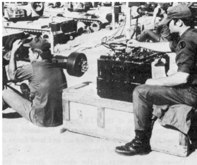
Dragon operator tracks a target vehicle downrange. Data collector to his rear monitors operator's performance and feeds incidental information into the computer.
