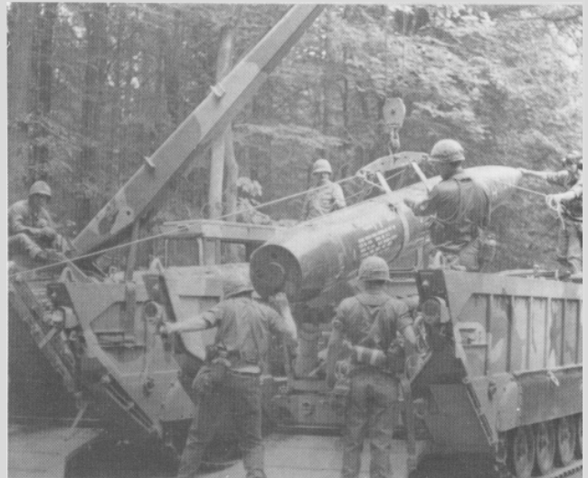
Figure 5 — Rapid Transload of Second Missile. As soon as the first missile is fired the loader transporter is moved to an open area and configured for a rapid transload while the launcher is enroute. A second missile is quickly loaded onto the launcher.
