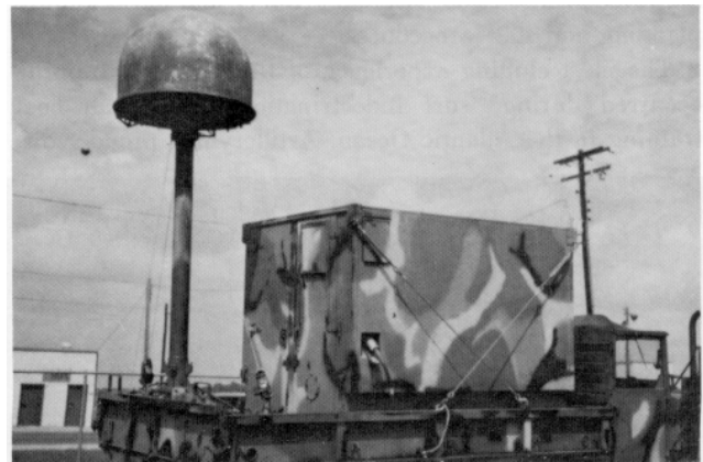
New vehicular configuration—TPS-25 mounted on 2½-ton truck.
