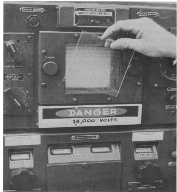
Figure 5— The plexiglass screen is removed from the trainer with the target echoes marked in grease pencil and is placed over the window of the radar. (Note: The trainer screen is designed to fit in the window of the radar and has a handle attached which allows it to be easily removed from the trainer and placed in the radar and vice-versa.) When the screen is placed in the window of the radar, the student aligns the strobe lines on the target echoes and reads the weapon location from the radar's computer.
