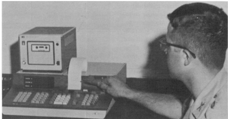
The computational unit displays the control point number assigned to the point of interest, the UTM Grid Zone, the Easting, Northing and height in meters in five to seven seconds.
