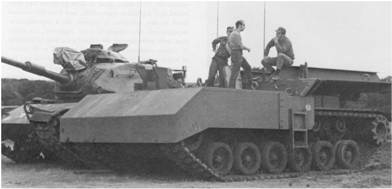
In the foreground is an M48A3 target tank used in HELBAT IV. The turret has been removed and replaced by 1¾-inch armor plate. In the background is an M60A1 tank used in a subexperiment of HELBAT IV.
