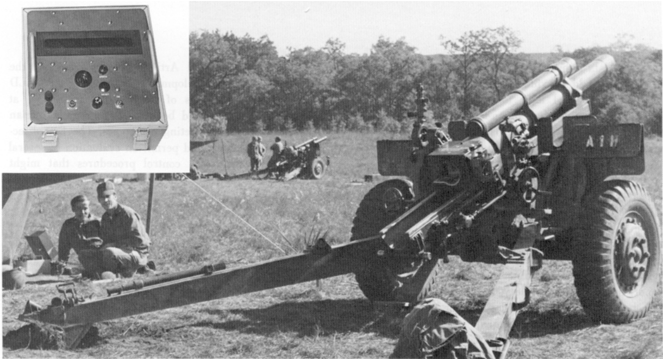
HELBAT IV howitzer section during a break in firing. Inset upper left is the weapon section data display unit that provides charge, deflection, fuze setting, and quadrant to the howitzer section.
