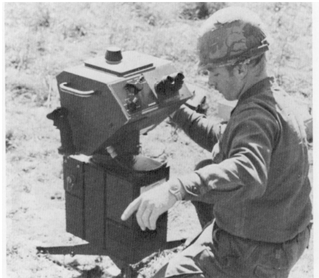
Ground laser locator designator (GLLD), one of two competing advanced development prototypes used in HELBAT IV.
