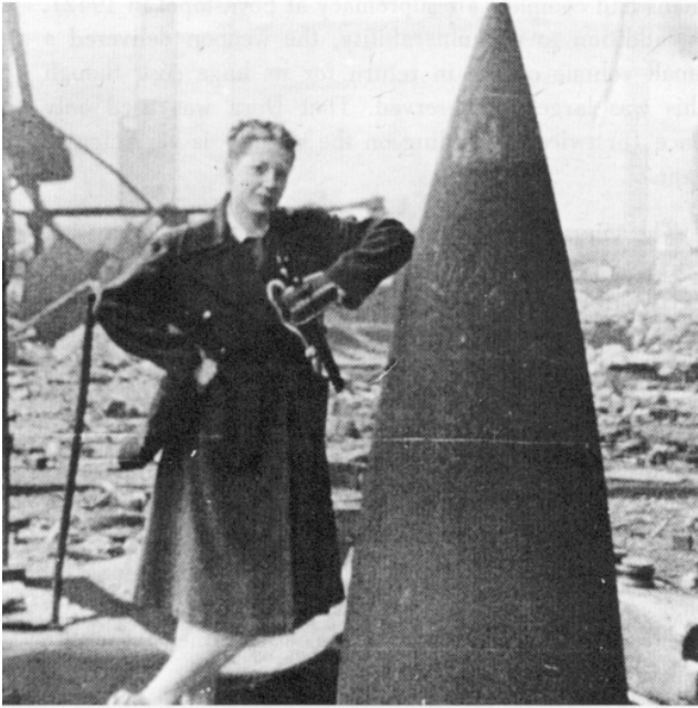
This 6-foot ballistic windshield (ogive) was used to protect the fuze from premature detonation.
