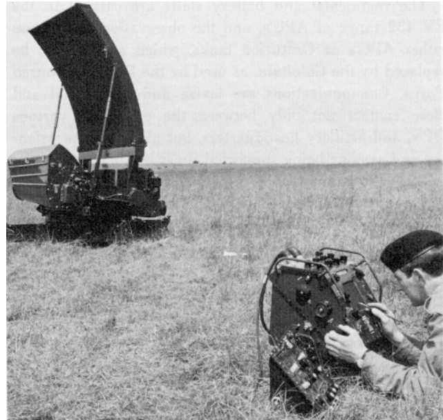
The Cyberline Mortar Locating Radar is slated to replace the Green Archer.
