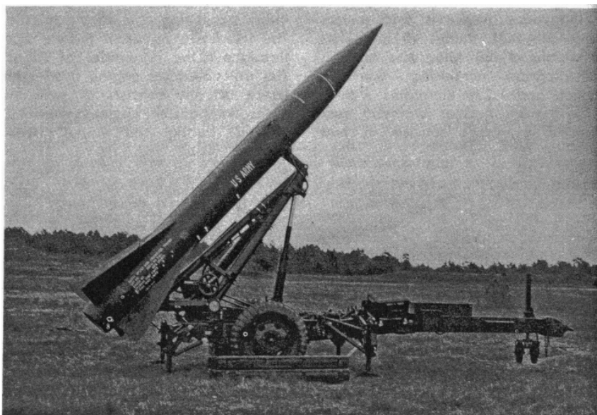
Launcher, zero length XM740
