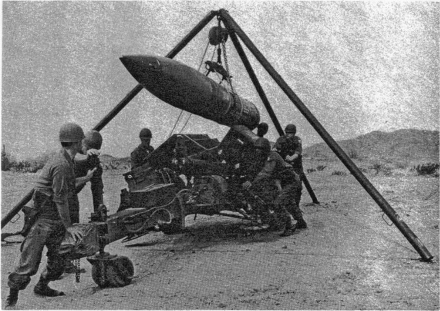
A hoisting unit tripod being used to load a missile on the LZL.
