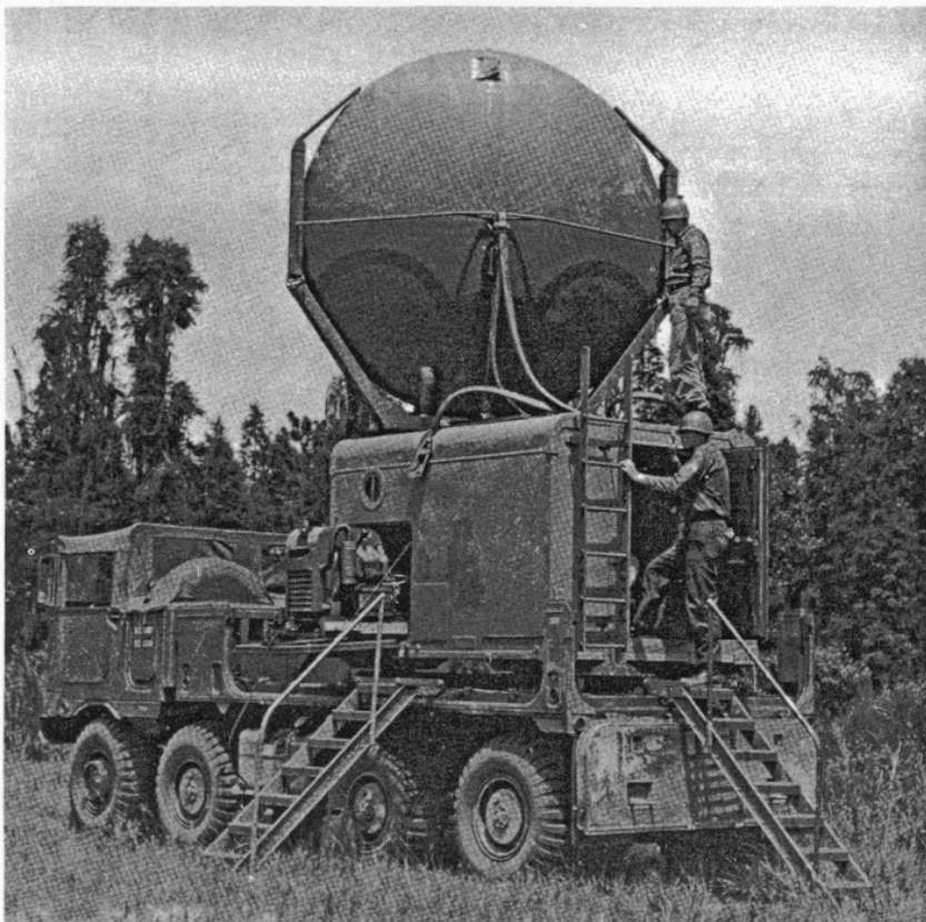
Figure 5. Being emplaced for action is the radio terminal set AN/TRC-80, with its 8-foot parabolic antenna. The communications set is transported on the new M656-series vehicle and is used in the battalion to battery communications link.
