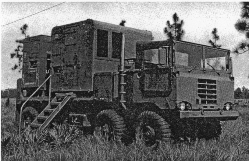
Figure 3. The Pershing 1a improved programmer-test station (PTS) programs the trajectory of the missile, controls the firing sequence, performs tests that simulate post-launch missile operation, and provides the operator with a visual indication of the firing sequence. To the rear of the PTS is the power station, which supplies electrical power, conditioned air, and high pressure air to the missile and ground support equipment during the countdown.
