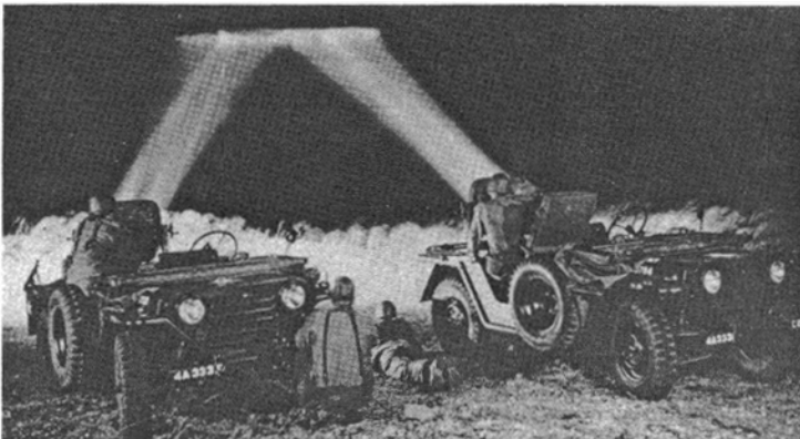
Figure 2. Jeep-mounted 23-inch xenon searchlight.
