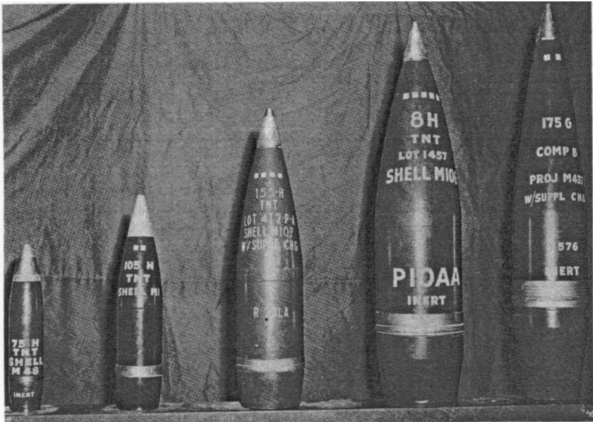
Figure 21. Comparison of U.S. Army Artillery projectiles
