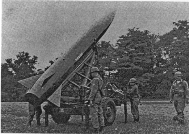
Figure 1. The Lance weapon system. The Lance is designed as a division support system. It marks the first use of prepackaged liquid propellants by the Army. When fielded, it will have all the reliability and simplicity of free rockets and an increased range and accuracy normally associated with guided missiles.
