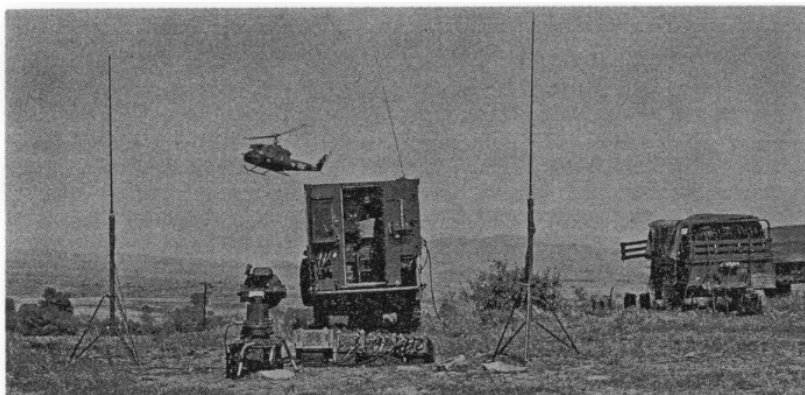
Figure 8. Ground station control equipment including shelter-mounted computer, tracker, distance measurement equipment, and power generator. Airborne station mounted in co-pilot's door of UH-1B.
