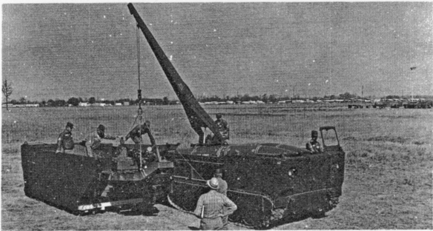
Figure 5. Firing unit is removed from self-propelled launcher. the full mobility adaption kit. The lightweight launcher may be towed by a prime mover with a capacity of 1 ton or greater. The launcher platform may be traversed and elevated manually.
