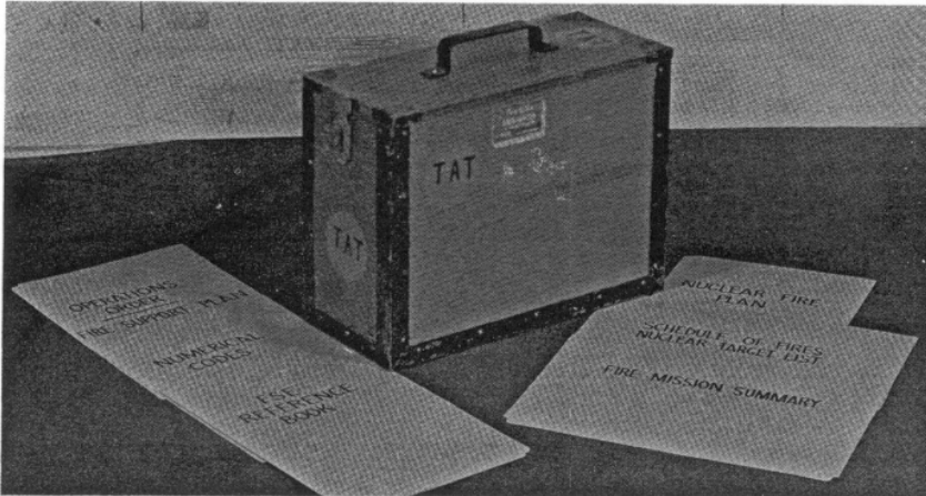
Figure 6. Metal reinforcements on the corners protect structure. CONUS units should mark box as yellow disk TAT.
