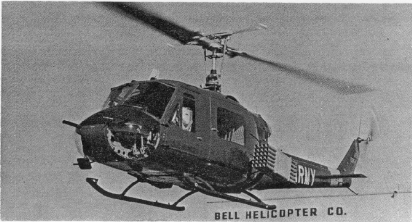
Figure 5. XM3 (UH-1 helicopter with 2.75-inch rocket pods attached).
