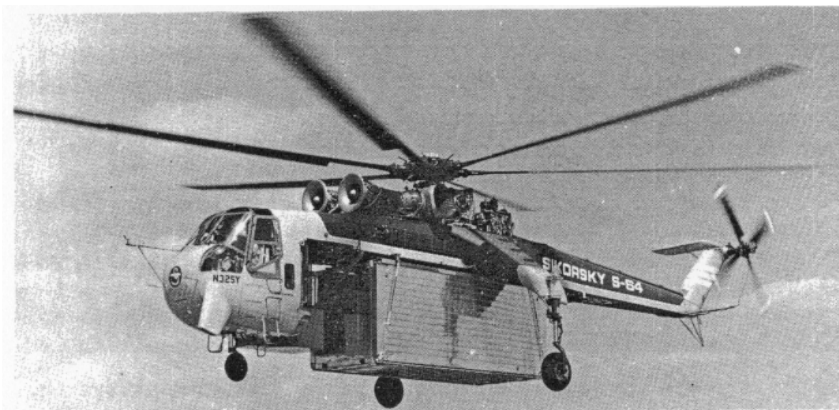
Figure 6. Experimental "sky crane": 8,000 horsepower, 10-ton lift capacity.
