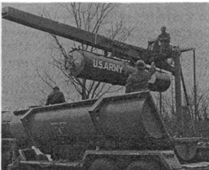
Figure 16. The launching station is leveled, and the boom is unfolded to the loading position. Left.
