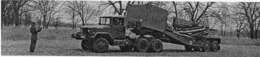
Figure 14. The Sergeant can be assembled and fired from a predetermined position with nine crew members. The launching station can be emplaced in an area as small as 20 meters in diameter.
