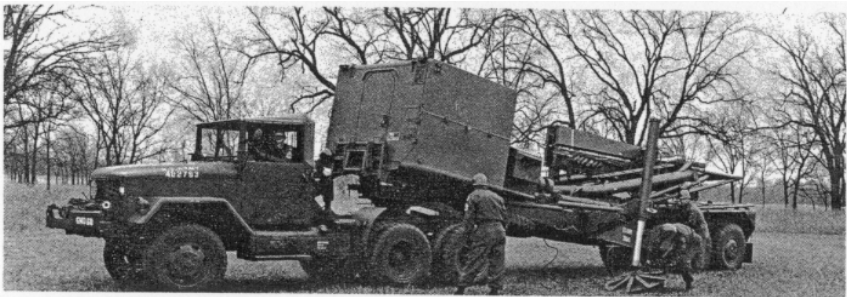
Figure 15. The power generator of the Sergeant is started, and then the outrigger jacks are lowered on the station, which provides the assembly and firing platform for the missile.
