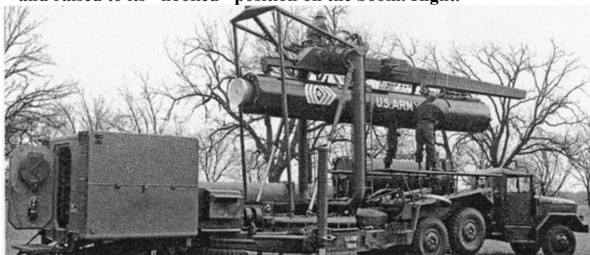
Figure 18. The guidance section of the Sergeant is removed from its container and attached to the rocket motor with four bolts.
