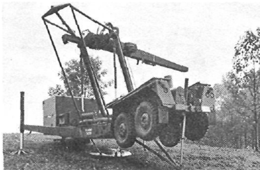
Figure 3. Launching station: length 31 feet 3 inches; weight 17,000 pounds. Used to assemble, erect, program, orient, and automatically launch the missile.
