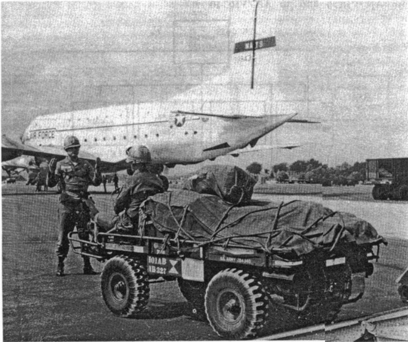
Figure 29. The M274 carrier has a payload of 1,000 pounds.
