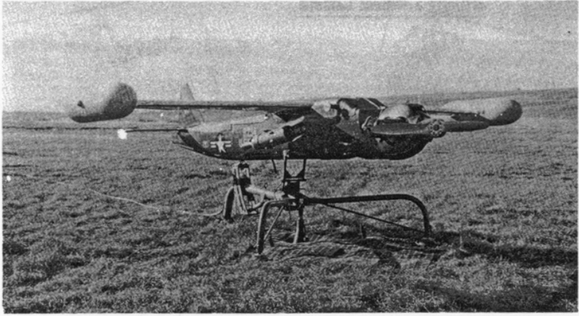
Figure 1. The SD-1 drone ready for takeoff on its zero-length launcher.
