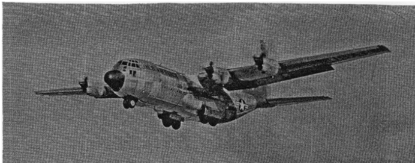
Figure 11. The C-130 aircraft has four turboprop-type engines.
