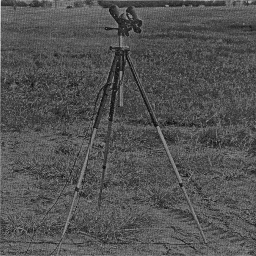
Figure 26. Skyscreen equipment of the Lacrosse trajectory safety system.
