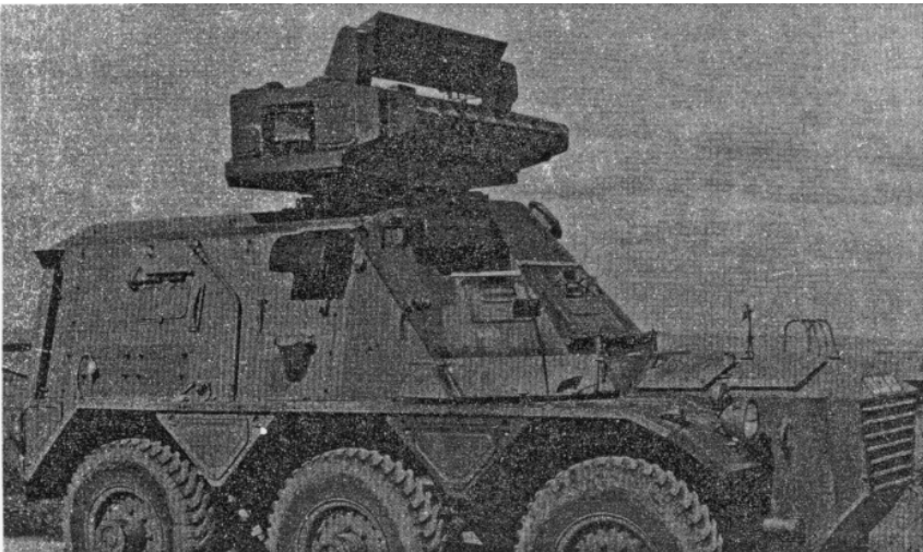
Figure 13. General support radar nr 9, MK1.
