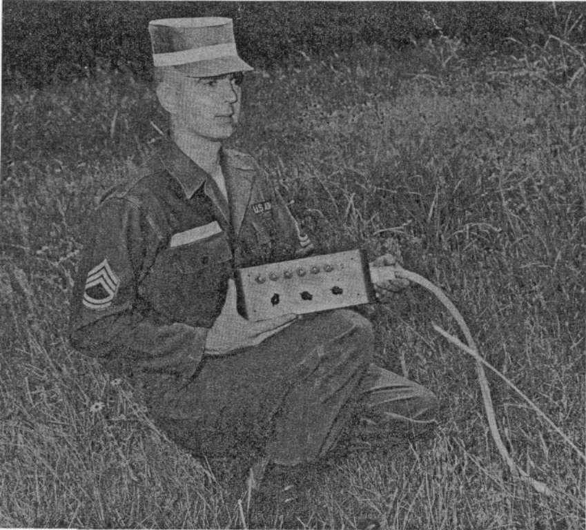
Figure 23. The instructor's console, heart of the Lacrosse handling and checkout trainer.
