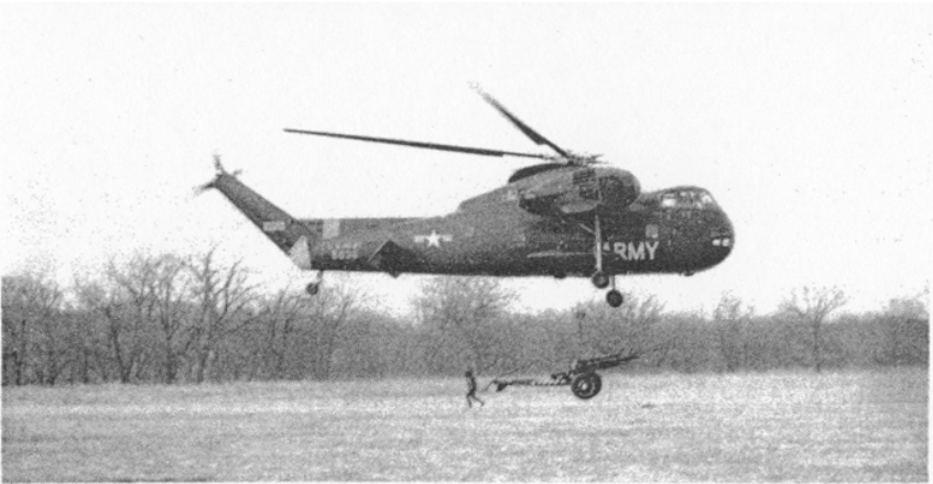
The hookup man signals the pilot that the howitzer is secure in the sling and ready to move out.
