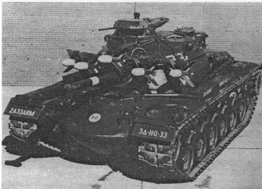
Figure 36. SS10 antitank guided missiles mounted on the M48 tank.
