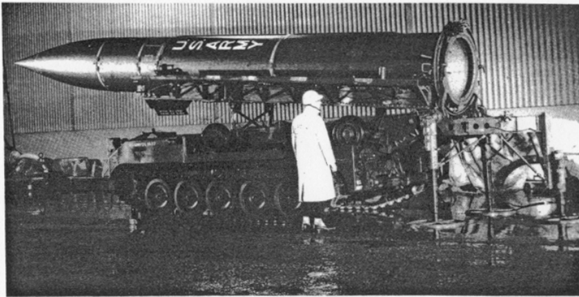
Figure 16. The Pershing on its transporter-erector-launcher which is mounted here on the XM474 track vehicle. Note the launching platform already on the ground at the rear of the vehicle.
