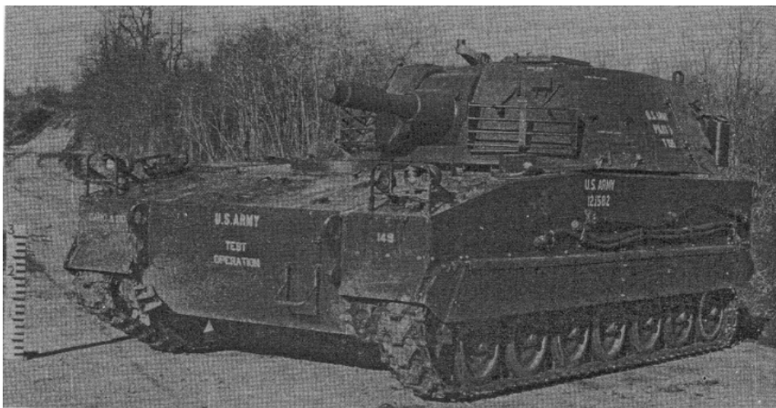
Figure 27. The T195 self-propelled 105-mm howitzer is an armor protected, full-tracked vehicle.
