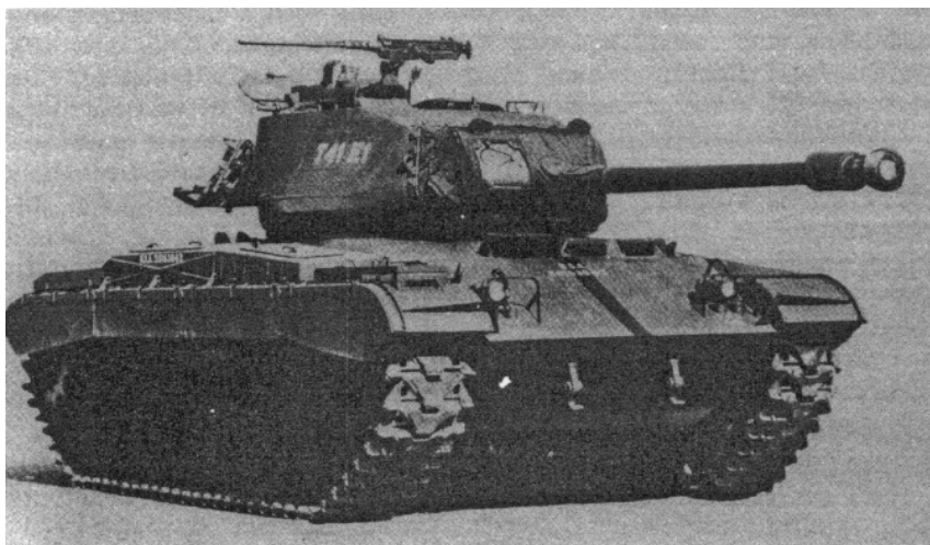
Figure 22. The M41 light gun tank, popularly known as the "Walker Bulldog," is the basic fighting vehicle of the armored cavalry regiment.
