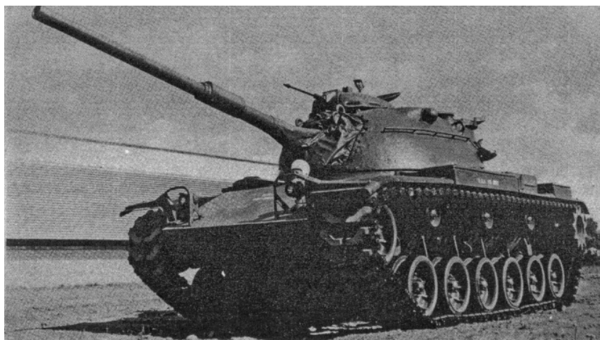
Figure 25. The M60 medium gun tank boasts a 105-mm gun and diesel power.
