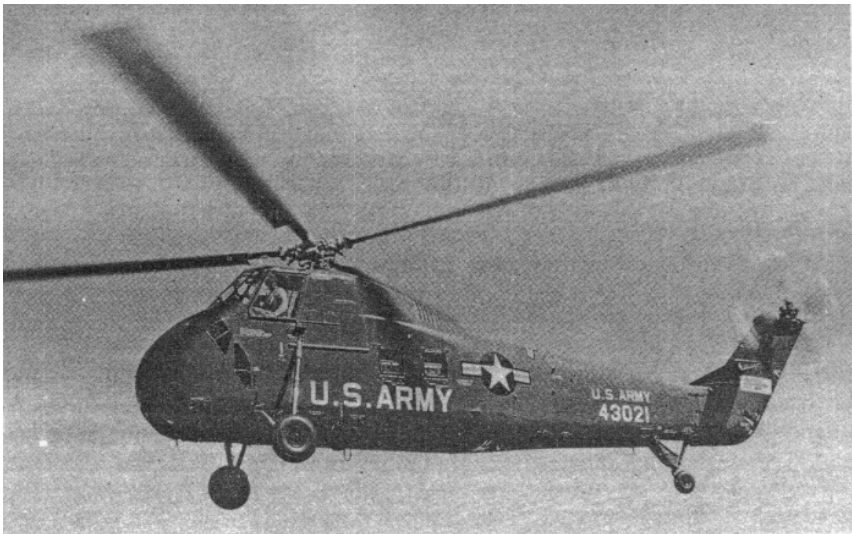
Figure 53. The H-34, Choctaw, is powered by a 9-cylinder radial piston engine.
