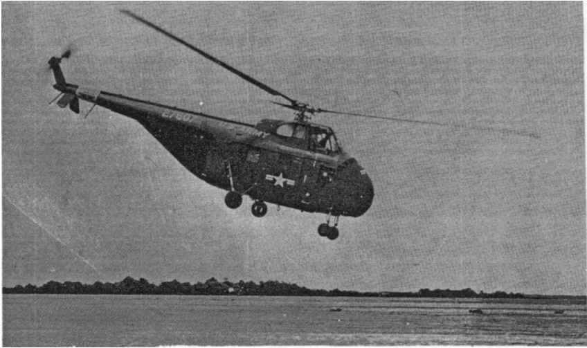
Figure 50. The H-19, Chickasaw, has a range of 200 miles.
