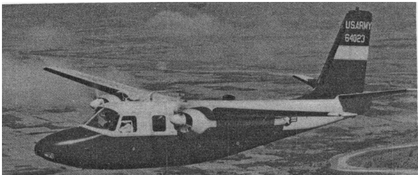
Figure 56. The L-26 has a total rating of 680 HP.
