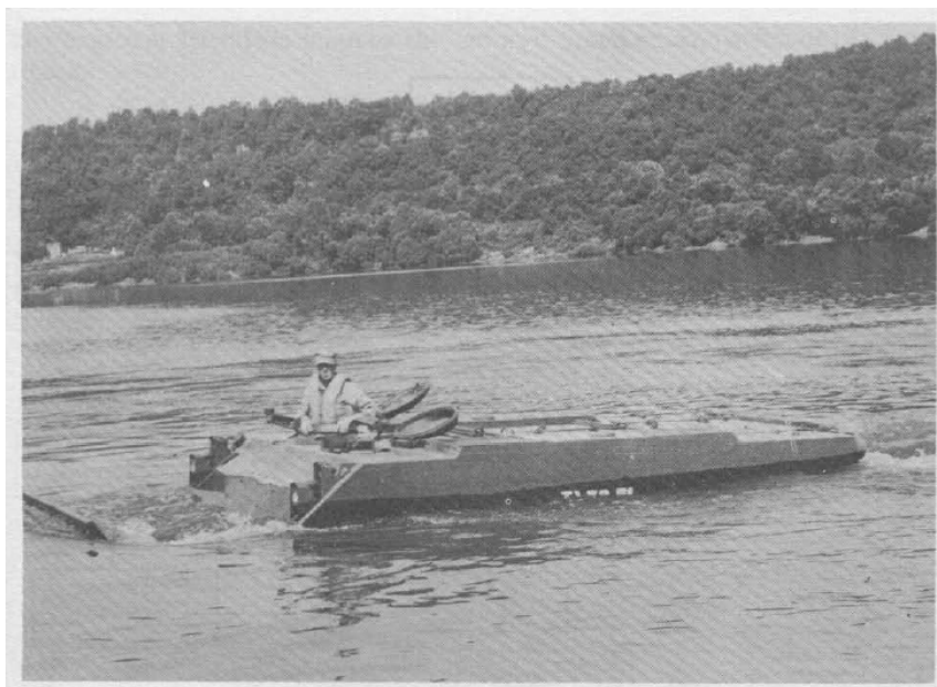
Figure 23. The M59 armored personnel carrier has all-around armor protection and is amphibious.
