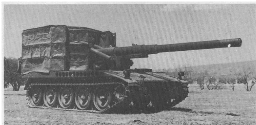
Figure 37. The nylon cab is shown on the 155-mm gun, T245. It is being tested concurrently with the plastic cab.
