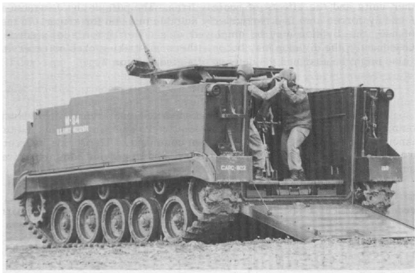
Figure 20. The 4.2-inch mortar is fired from the M84 armored mortar carrier.
