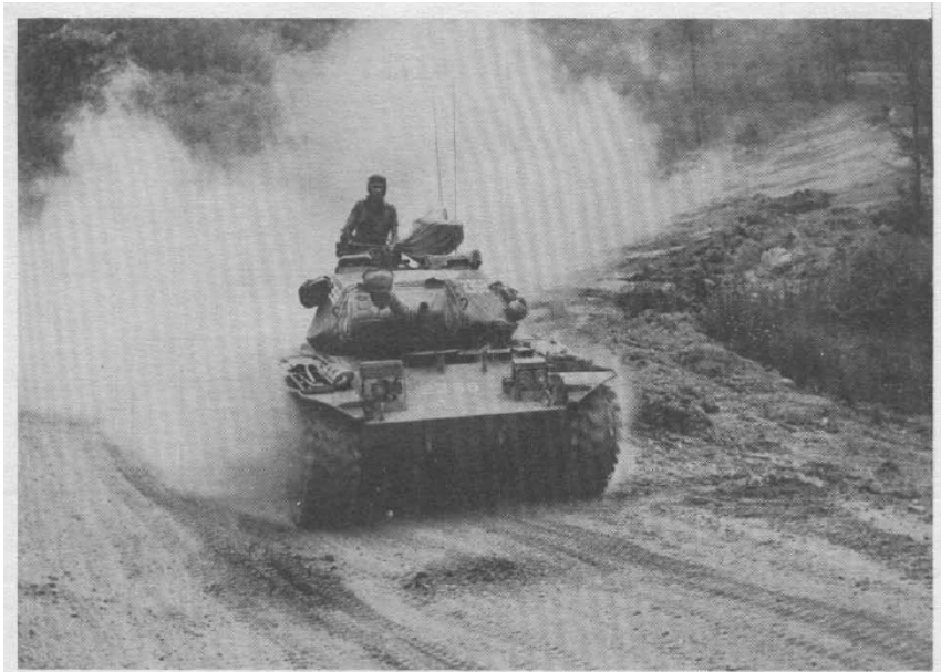
Figure 25. The M41 light tank, or "Walker Bulldog" has a 76-mm gun.
