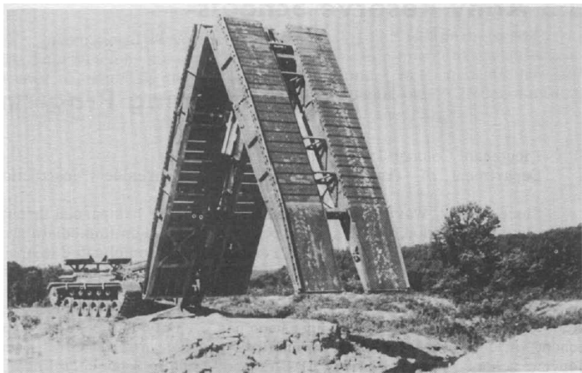
Figure 27. A bizarre piece of equipment, the self-propelled armor bridge.
