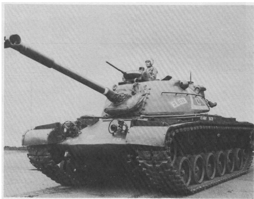
Figure 21. The M48 medium tank, popularly known as the Patton tank, has a 90-mm high velocity gun.
