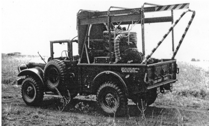
Figure 40. The XM387, hydrogen peroxide servicer, carries a 78-gallon drum of concentrated hydrogen peroxide which is used to generate steam to operate the missile's propulsion system. The propellant loading sequence is: alcohol, LOX and hydrogen peroxide.
