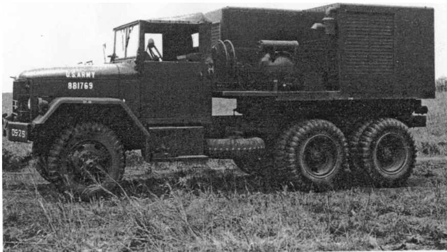
Figure 36. The truck-mounted air compressor provides 5,000 pounds per square inch of air pressure. During flight the compressed air, which is stored within the missile, is used to pressurize the alcohol and hydrogen peroxide tanks and to open and close valves in the propulsion system.
