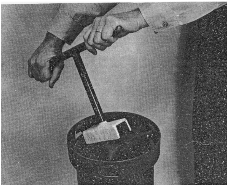
Figure 49. The wrench being used to open an 8-inch howitzer powder bag container.
