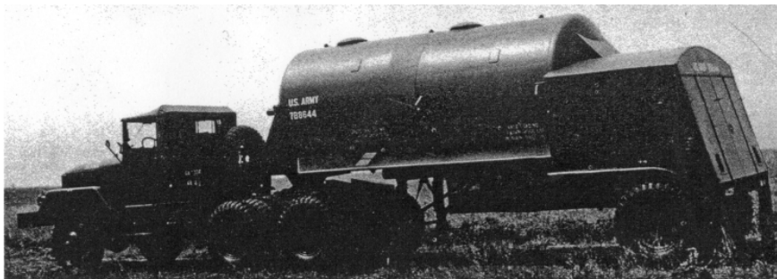
Figure 39. Each firing battery has two liquid oxygen (LOX) semitrailers that carry the oxidizer to service the missile. Each trailer can hold 9 tons of LOX. The trailer has a "thermos bottle" construction to maintain the LOX at a temperature of minus 297 degrees Fahrenheit. The LOX transfer pumps and equipment are mounted in the closed compartment at the rear of the trailer.
