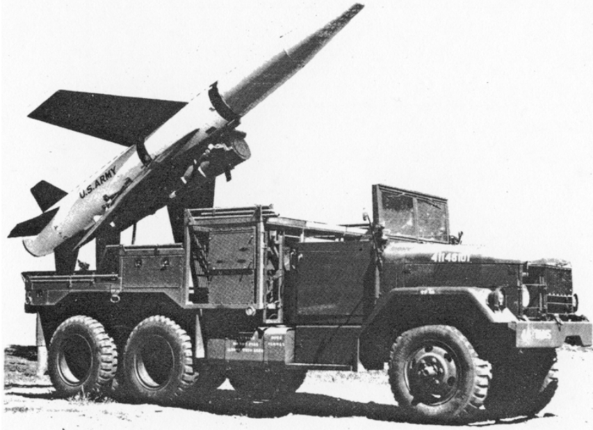
Figure 5. The Lacrosse is launched from a 2½-ton truck.
