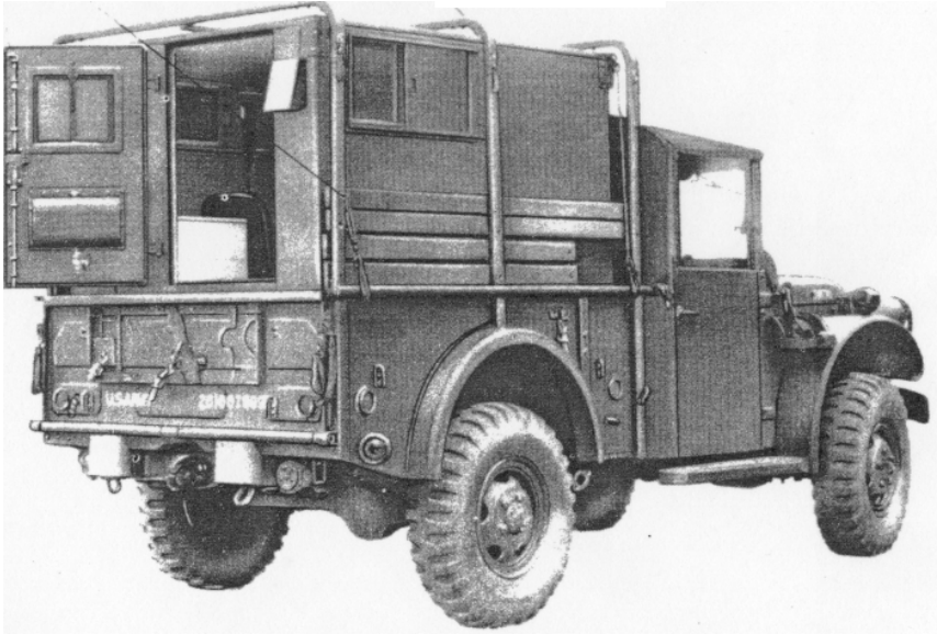
Figure 19. The shelter mounted on a 3/4-ton truck. Its power source is the vehicle's electrical system.
