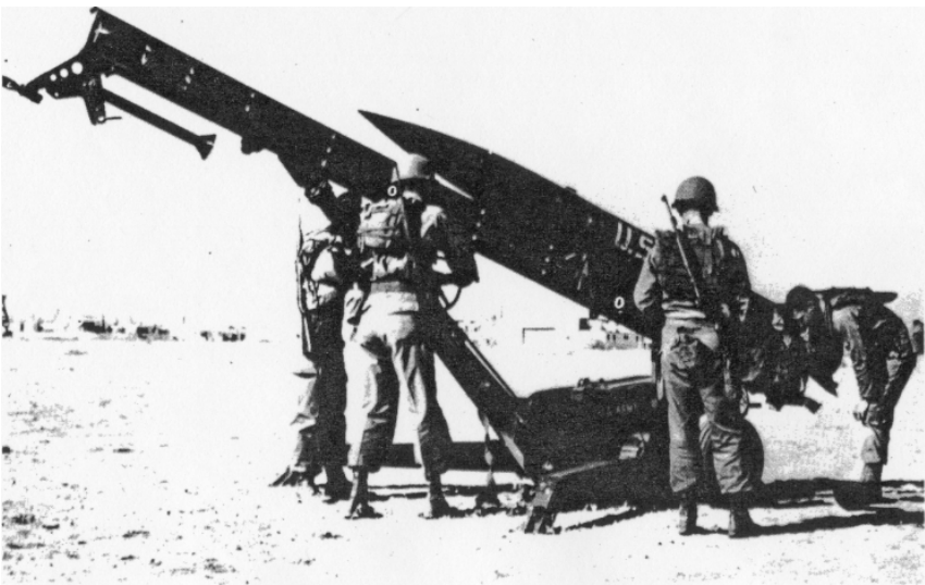
Figure 4. The Little John shown here on its launcher is undergoing a prefire checkout.
