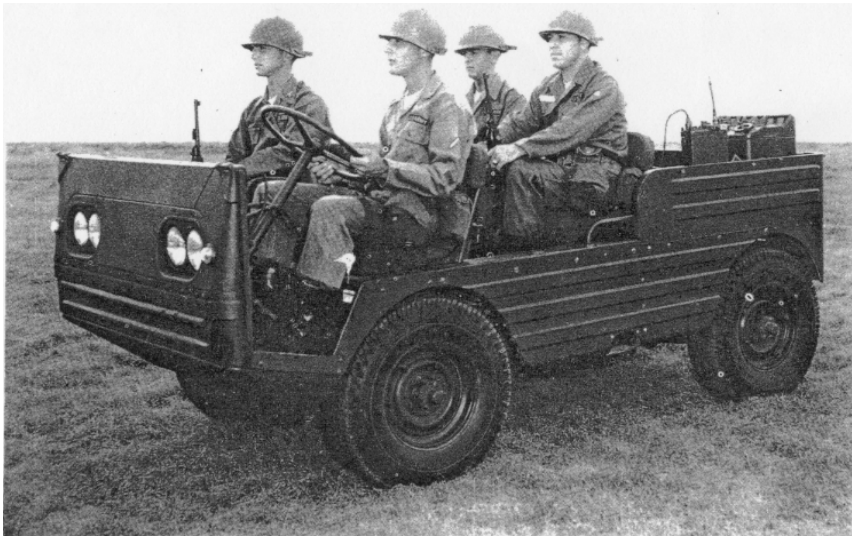
Figure 22. Side view of XM443 E-1 illustrates the vehicle's low silhouette and the ease with which passengers can mount and dismount.
