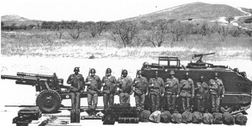
Figure 15. A second possible use for the T117 is as a prime mover for the 105-mm howitzer.
