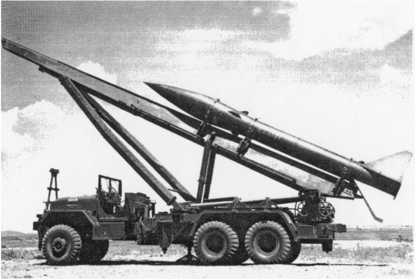
Figure 3. The Honest John and its launcher mounted on a 5-ton truck.
