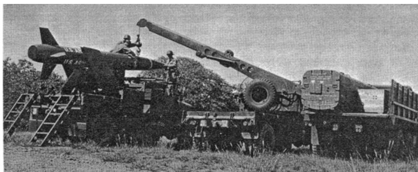
Figure 10. The 2½-ton wrecker is used to transfer the missile and warhead from the ammunition truck to the launcher. This sequence shows the warhead being mated. The warhead is removed from its container with a nose handling eye.
