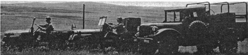
Figure 4. The preceding photographs have shown the Lacrosse guidance equipment ground-mounted. The equipment also may operate from the section's vehicles, shown here in traveling position, except for the angular tracker which must be operated from the ground.
