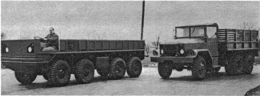
Figure 39. The XM410 (left) is shown with a standard M35 2½-ton truck (right).
