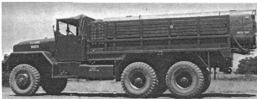
Figure 8. The 5-ton cargo truck can carry 2 complete missiles in their containers.
