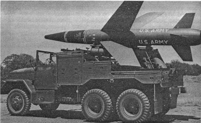
Figure 5. The Lacrosse can be transported on its 2½-ton truck-mounted launcher with the wings off (top) or with the wings mounted (bottom).
