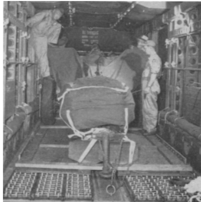
The PEGASUS. Fairchild Engine and Airplane Corp. 105mm M2 in a C82. A jeep is in front of the howitzer. Note rollers under platform.
