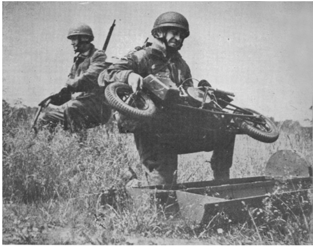
British paratroopers assemble folding motorcycles ("Wellbikes"). Light and speedy (40-45 mph), they drive on rough terrain, getting 180 miles per gallon of gasoline.
