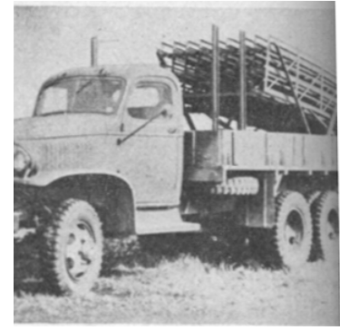
This T-32 launcher fires 7.2" rockets.
