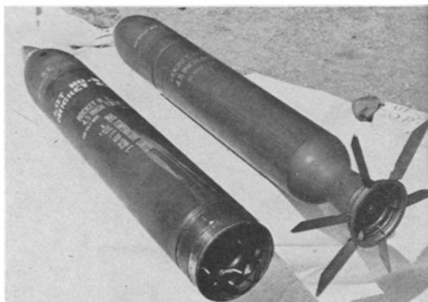
Another study of the two methods of stabilization as illustrated with the M16 and M8 rockets.
