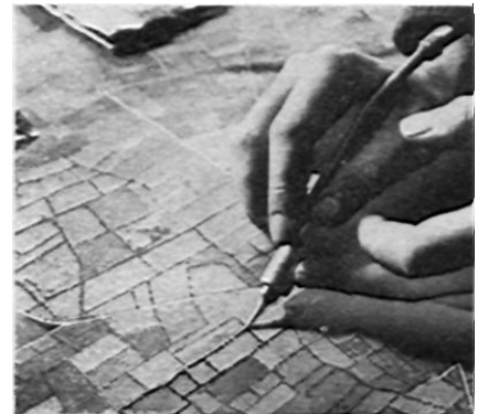
Applying trees and hedges with a compressed extrusion gun
