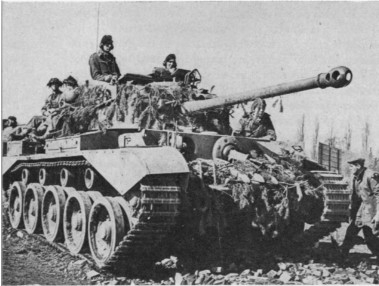
Descending from the "Cromwell" tank which proved itself in the British advance through France and Belgium, this "Comet" is Britain's fastest and most heavily armored cruiser tank. It is powered by the Rolls Royce "Meteor" engine and carries a 77-mm gun with a new laying device which greatly increases accuracy. From the Rhine to the Elbe and beyond the "Comet" led the British advance. In this picture a "Comet" of the 11th Armoured Division moves up on the Weser bridgehead in April, 1945.
