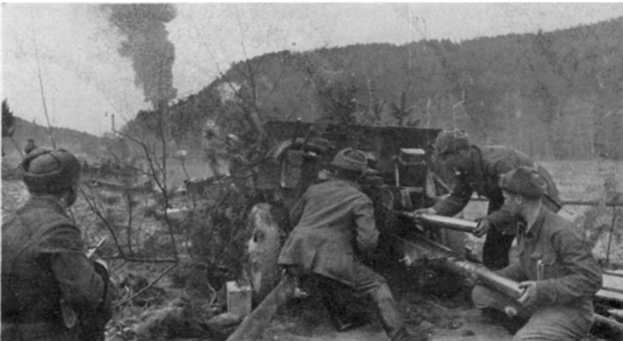
Two views of a very rare Russian piece, the 76-mm antitank gun. In the upper photo the round is a standard AP-HE; its new case probably gives a muzzle velocity of 2,600-3,000 f/s.
