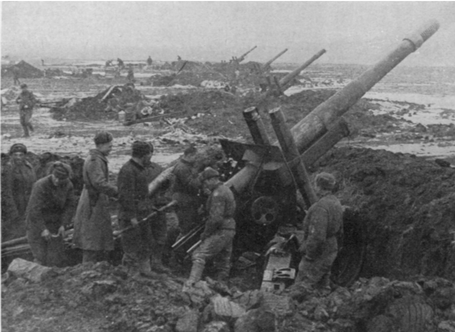
Fitted with muzzle brake, the Russian 152-mm heavy field howitzer fills the same role as our 155-mm howitzer. M1. It has a Schneider flavor throughout.
