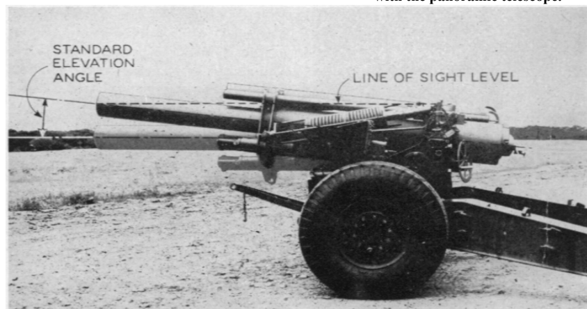
Figure 18. Tube elevated until pin on muzzle is level with optical axis of panoramic telescope.
