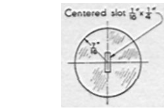
A dark colored cardboard or metal disk of the same diameter as the aiming circle eyepiece lens focusing sleeve.
