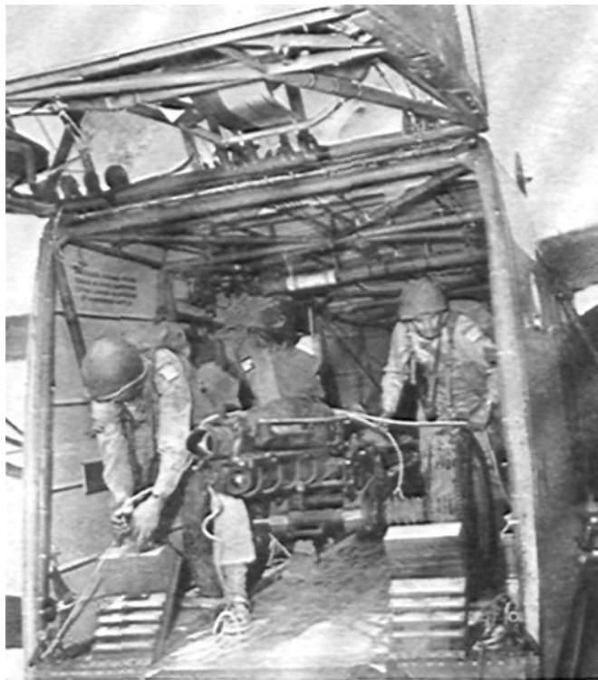
For airborne operations, all equipment must be well braced and lashed. This 75-mm howitzer belongs to the 82nd Airborne Division.
