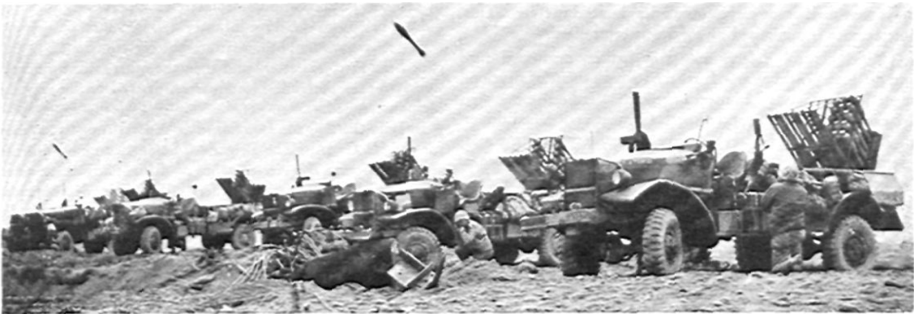
Saipan saw the Marines' first use of mobile rockets. These truck mounts were ideal for two Jima—hit-and-run tactics prevented the Japs from getting a fix on their positions.
