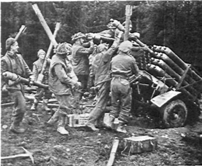
For barrages, 12 of these British 32-barrelled projectors are used together. Resultant fire power is similar to that of 280 5.5" guns (which fire 100-lb. shells), but a rocket battery needs less than 200 men.
