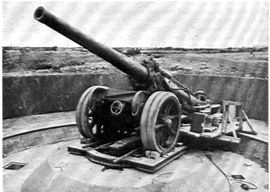
Here is a circular emplacement found on the French coast. Although big, cumbersome, and hard to camouflage, such an installation does facilitate fire control and may increase the accuracy of laying. The piece shown here is a French 155-mm gun. St. Chamond, model 1916 (called by the Germans the 15.5-cm K.420 (f)). It is 38 calibers long and has a maximum range of around 22,000 yards; its traveling weight is 13,090 kilograms—about 14½ tons. For stability in normal firing the carriage is braced by two jacks; these are emplaced by means of handwheels, one of which can be seen between the carriage wheels.
