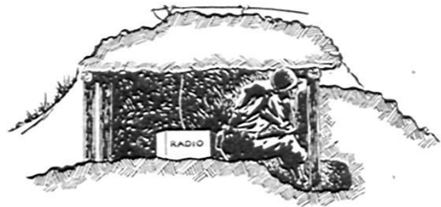
Figure 13. OP dug through crest of hill from reverse side.
