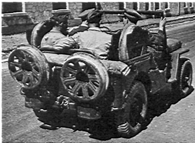
Our jeep has been adapted for railway use! When on the road, four trolley wheels are carried in special brackets without restricting the passenger space. For use on rails the wheels are changed, a clamp on the front axle holds the wheels straight, and a turntable device is brought into play at the point of balance under the transmission. This road-rail car should be useful for line inspection, and also for reconnaissance purposes.
