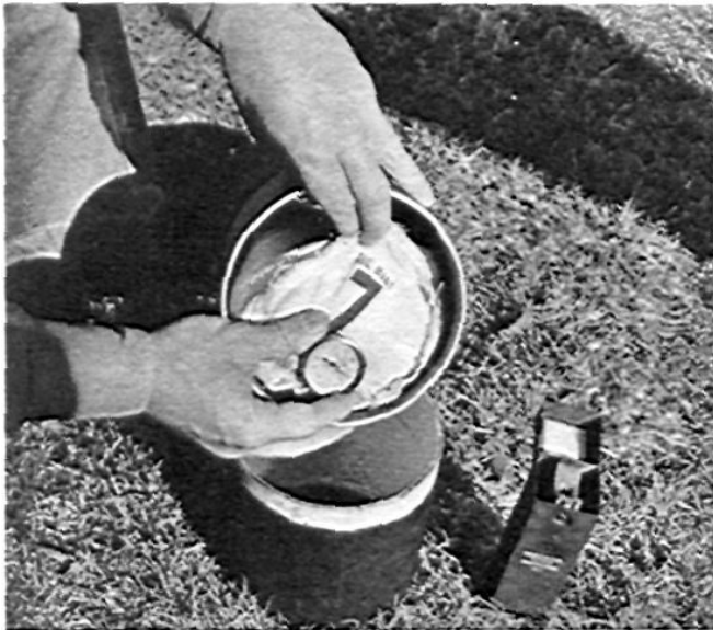
Powder Thermometer M-1, with propelling charge of separate-loading ammunition. After stem of thermometer is inserted in the bag, the charge (in its container) is stored under the same conditions as the balance of the ammunition.
