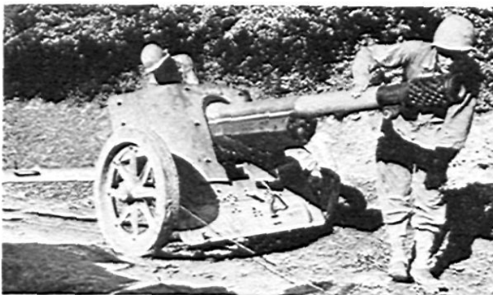
Germany's ingenious adaptation of captured materiel is well illustrated here: a Czech muzzle brake on a French 75 on the carriage of the German PAK 38 (5-cm AT gun), in the combination known as the PAK 97/38.
