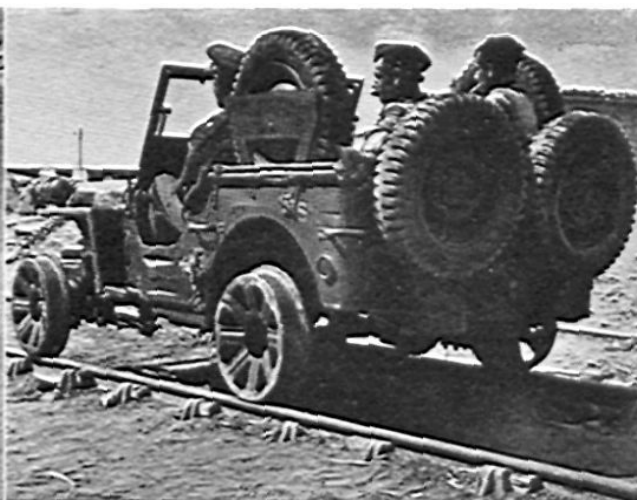
Our jeep has been adapted for railway use! When on the road, four trolley wheels are carried in special brackets without restricting the passenger space. For use on rails the wheels are changed, a clamp on the front axle holds the wheels straight, and a turntable device is brought into play at the point of balance under the transmission. This road-rail car should be useful for line inspection, and also for reconnaissance purposes.
