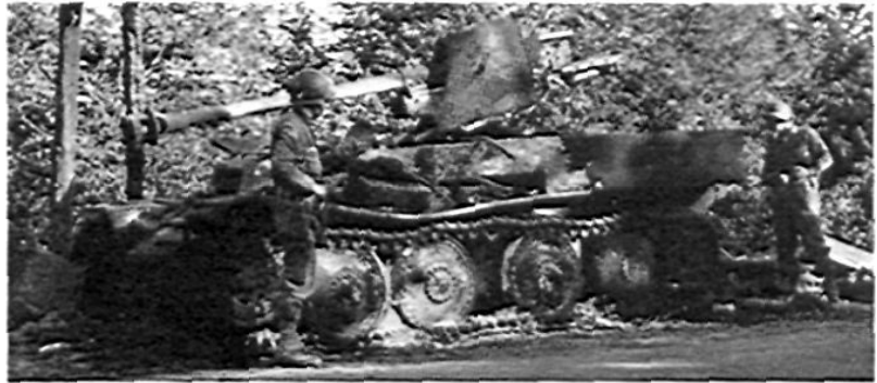
Well-placed AT fire has just knocked out (in Normandy) this German tank, which is being examined cautiously by alert GIs. This is a Russian 76.2-mm gun mounted on the PzKw 38 (ex-Czech) chassis.
