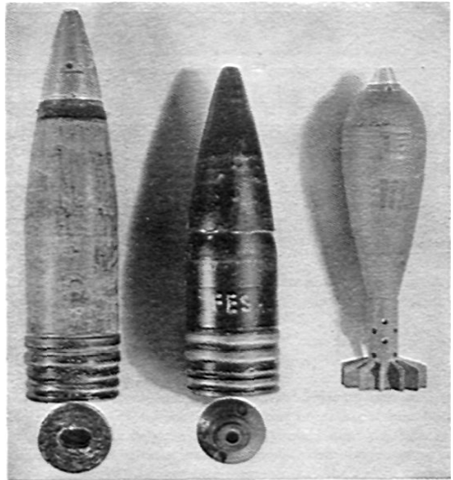
Figure 16. Three German shells of similar caliber but different type. Note closely differences in stamping, stenciling, openings, etc., which may aid identification after fragmentation. Left: 88-mm HE shell (German); AA and AT gun; projectile is filled from bore end. Center: 88-mm APC projectile (German); AA and AT gun; note base-detonating fuze and iron rotating bands. Right: 81-mm HE shell (German); S.G.R.W. (Schwerer-Granatewerfer) heavy mortar shell can be used in U. S. mortar.
