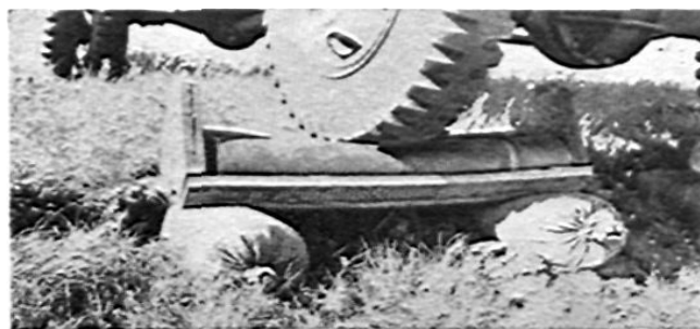
Figure 3. Test span indicating strength of dirt-filled ammunition containers in crate. Vehicle is a 1 1/2-ton truck.
