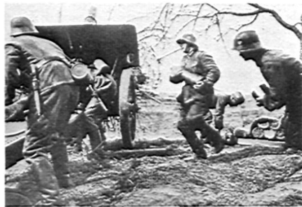
Reloading preliminaries: man at right has the charge in its short brass case, the next one carries a 1914 pattern short shell.
