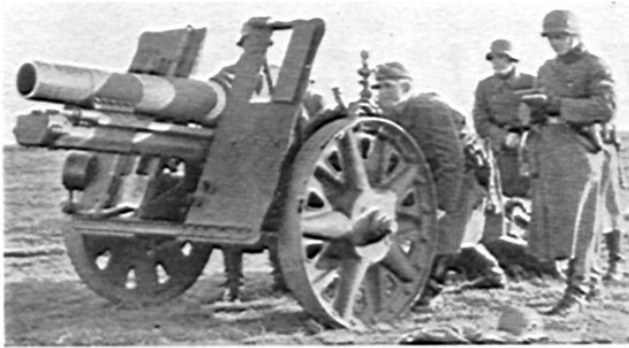
S.I.G. 33, 15-cm heavy infantry howitzer, is NOT a weapon of the type discussed in this article, although in its own way and within its limitations it is a quite effective piece.
