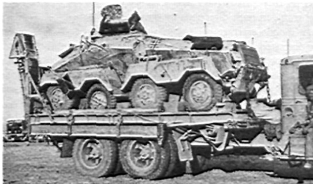
A 4 or 5 man crew (2 drivers, 1 or 2 gunners, and car commander) runs this 10-ton German armored car. The vehicle has dual steering control (fore and aft) and 8-wheel drive; 17½' long, 8' wide, and 9' high, it weighs 9 to 10 tons. Its turret revolves. Armament includes a light and a heavy machine gun. Notice how the body's armor plate is sloped to make bullets tend to ricochet instead of penetrate.
