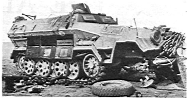
Standard German half-tracks have their plate sloped like that of the armored cars. Advantage is taken of the space thus provided to build in lockers for supplies. Like all other vehicles in the desert, this one carried fuel for warmth during the cold night or for cooking.
