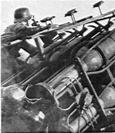
Germany also uses her 320-mm rocket in a carriage similar to that of a field gun. Six (or perhaps 8, in some cases) rockets are removed from their crates, put in guides on the carriage, and fired electrically.
