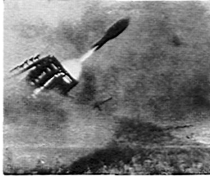
Germany also uses her 320-mm rocket in a carriage similar to that of a field gun. Six (or perhaps 8, in some cases) rockets are removed from their crates, put in guides on the carriage, and fired electrically.
