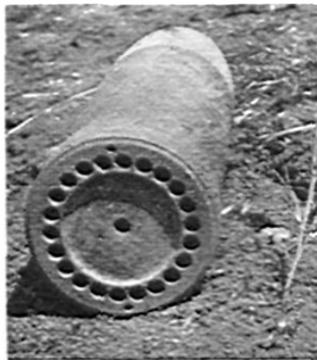
22 ejection holes for the 21-cm Nebelwerfer projectile form a closely-knit ring about its base.
