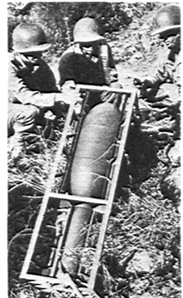
Details of the larger incendiary rocket appear here. Lattice-work crate contains guide rails for firing. The crude sight folds forward to prevent projectile from falling from crate during shipment. Officer at right seems to be holding a screw-plug removed from near nose of projectile; this is likely where the incendiary liquid is poured in.
