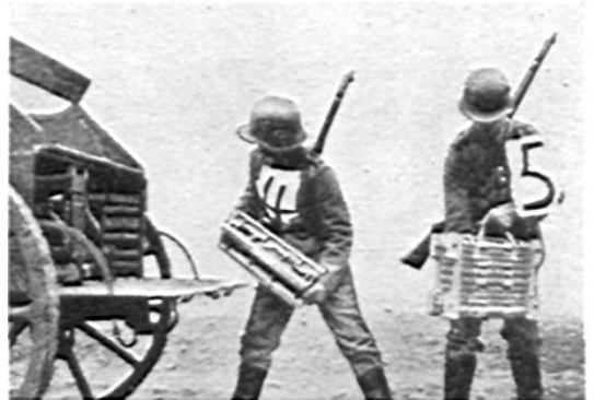
An I.F.H. 16 caisson is shown here with the new style (I.F.H. 18) shell crate and cartridge case basket. The crate contains one fuze HE shell. The basket carries 6 primed cartridge cases, each with increments for zones 1 to 6.
