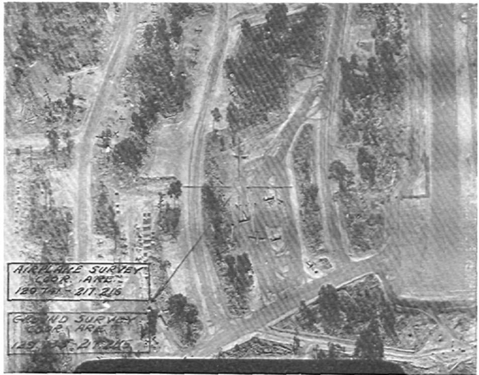
Example of "grasshopper" survey. In this particular test the airplane survey and the ground traverse differed by only 8 yds. on the X coordinate and 9 yds. on the Y.
