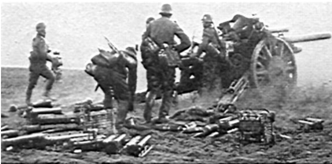
These pieces have the first pattern of pressed steel wheel, but with steel tires rather than rubber ones. In the left picture note the extreme litter of ammunition in the immediate vicinity of the piece; although the uncased projectiles are laid on canvas or paper, they are spotted where much sand and dirt will inevitably be kicked among them. At the right (a battery being fired at the Sportplatz in Berlin before this war) you can get a good idea of tube length, piece silhouette, and pattern of this type wheel.
