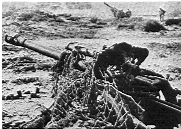
I.F.H. 18 M is the latest version of this weapon, fitted with muzzle brake so it will withstand the effects of higher muzzle velocity.
