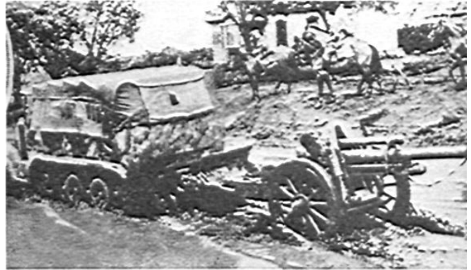
A variant appears here, on the Russian front. Prime mover is a standard personnel carrier. Wheels of the piece are the old wooden, steel-tired type, but with solid rubber tires mounted on them.
