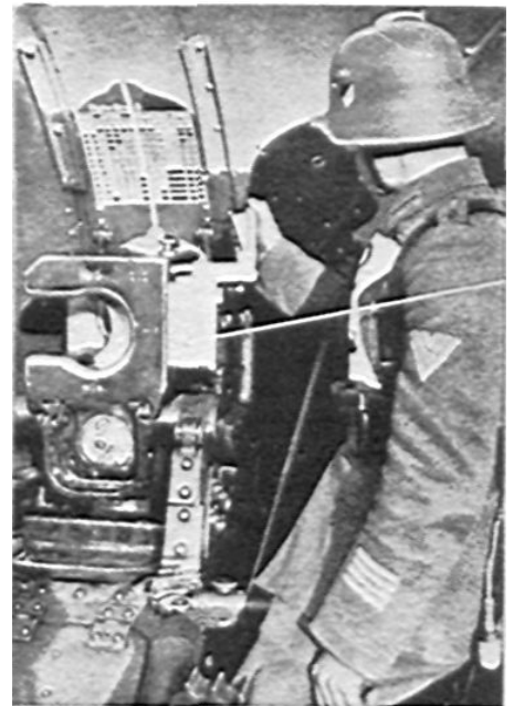
Pulling operating lever to the rear opens the block on this model. Note that here, as with practically all their artillery pieces, the Germans paint a skeletonized range table on the shield.
