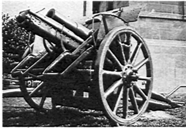
1.F.H. 98/09 was the first "modern" 10.5-cm howitzer. Its tube was extraordinarily short, but its modified box trail carriage was efficient enough to be retained in the 1916 version.
