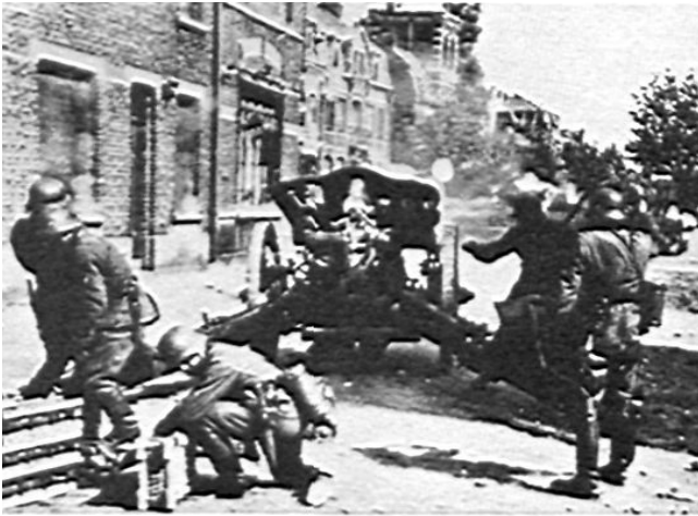
In a French street, Germans are firing a 10.5-cm howitzer fitted with steel-tired wheels.
