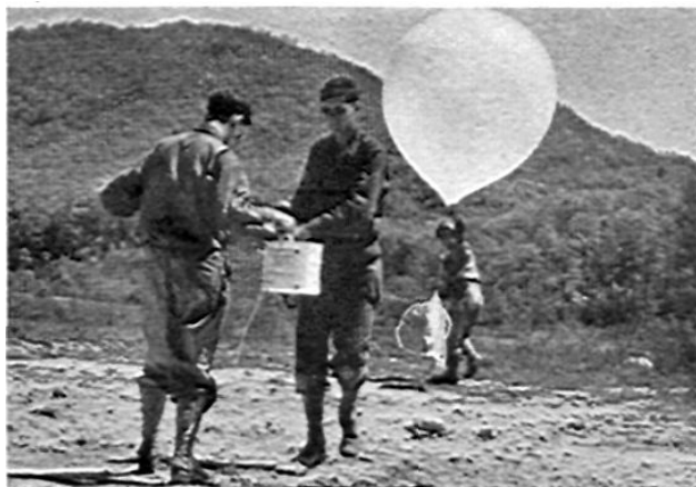
Two soldiers in foreground are holding a radiosonde, a 2-lb. box of instruments for measuring temperature, humidity, and pressure at upper air levels. It radiates a running record of this data for the various layers of atmosphere through which it travels. In background a soldier is about to release the balloon which hauls aloft the equipment and also a parachute which carries the delicate instruments back to earth.
