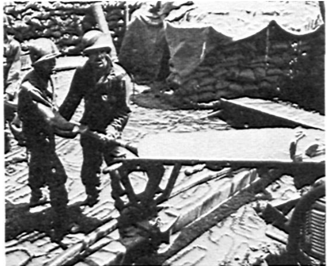
Loading tray must be long, to accommodate a 102-lb. bag of powder, as well as stout, to support the heavy projectile.
