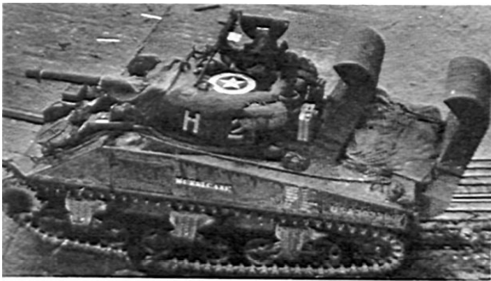
Tanks were especially waterproofed. In this particular case that was an unnecessary precaution, but with all openings well scaled and special intake and exhaust ports this vehicle was all ready for a wet landing. Notice that the waterproofing does not interfere with prompt use of weapons.
