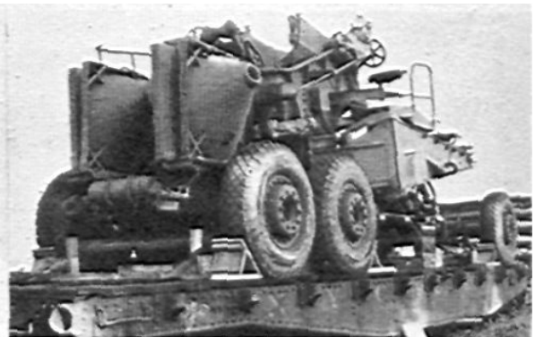
These pictures show the 240-mm howitzer and carriage M-1 blocked for rail transport.
