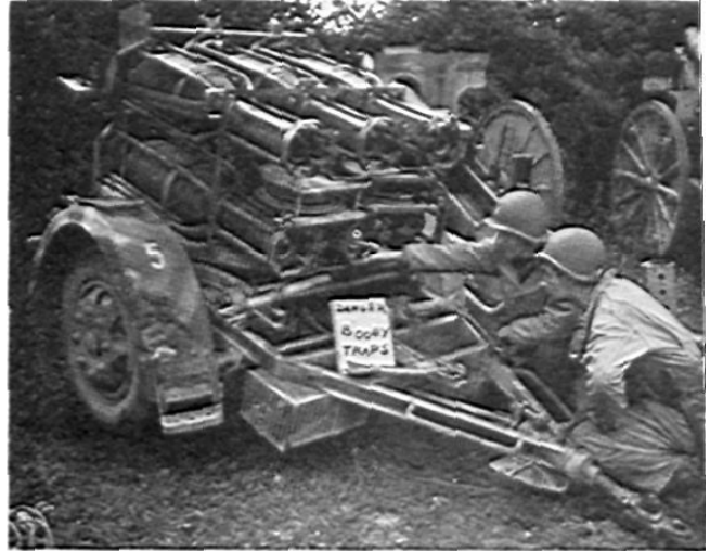
Soon too, much German equipment was captured. This rocket launcher is well placarded. Note the open, hinged metal cover which protects the rockets' intense heat and blast. At the right are a couple of 1935 French 105-mm howitzers—the ones whose wheels turn knock-kneed when the piece is emplaced, to provide, in effect, additional shields.
