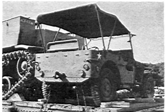
An alternate method of securing the 1/4-ton truck is to turn the vehicle crossways on the car by manpower, and secure by cleats and wires as shown here. By removing the spare wheel and gasoline can carrier, the overhang is reduced enough to pass railroad inspection.
