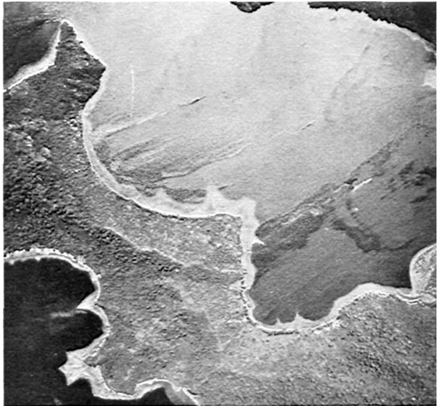
Reversing Lt. Craig's situation, a navy photographer made this photo from an army plane. Taken from 14,500 feet, it well illustrates how clearly island shorelines appear. Although detail in the interior is scanty, a careful study of water depths, plantations, and general growth will often (as here) reveal the major ground formations. Three Jap cruisers are in Buka Passage, at the upper right.
