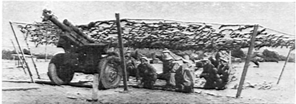
A firing embrasure is formed in corner of the net by dropping corner pole (No. VIII) and rolling net back to wire placed diagonally across corner.
