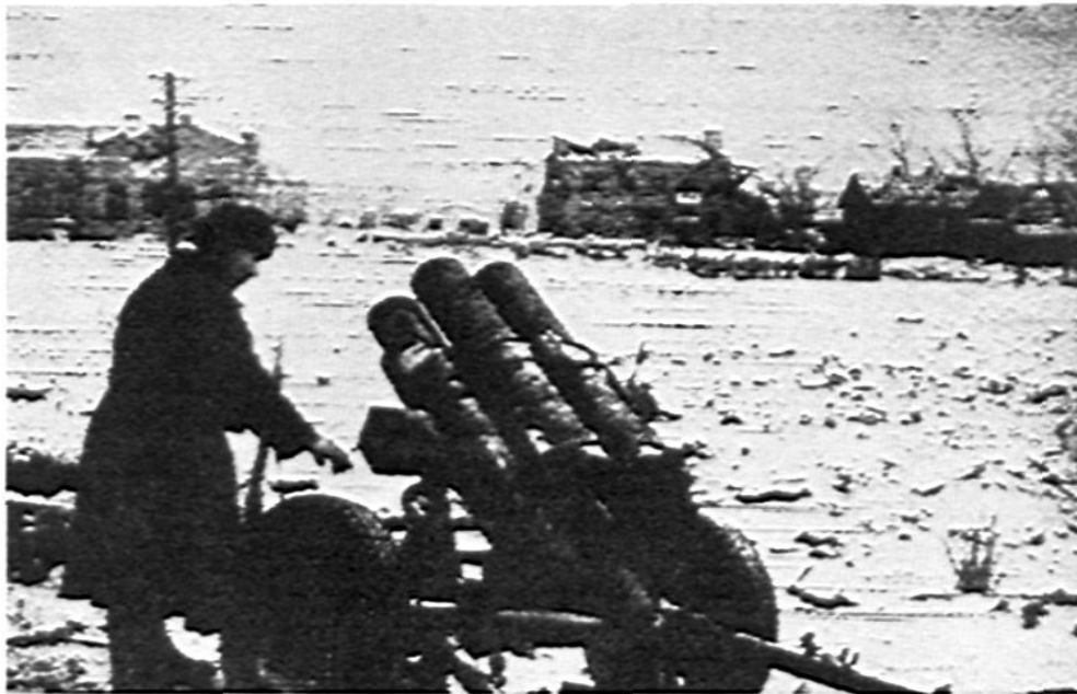
This German 6-barrelled rocket gun was captured at Veliki Luki. Caliber is 15-cm., and it fires a (roughly) 50-lb. projectile about 6,000 yards. Barrels are of course open at both ends, but each has a finger-like projection to hold rockets in place when tubes are elevated. Barrels contain 3 straight guide rails about 1/3" deep. Despite the absence of rifling, projectiles seem to rotate in flight—probably due to the set of their venturis. Firing is electrical, in rotation, at 1-second intervals. The whole assembly is called the Nebelwerfer 41.
