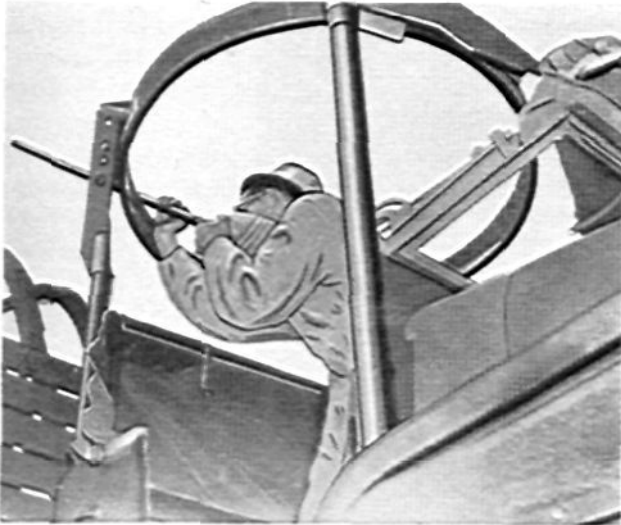
Fig. 4.—Sweeping the sky clear of enemy planes. To enable the assistant driver to fire at aerial targets, the seat cushion is taken out, the seat is thrown up, and he has a clear area of floor space to dance around on. The gun ring allows a machine gun to fire in all directions.
