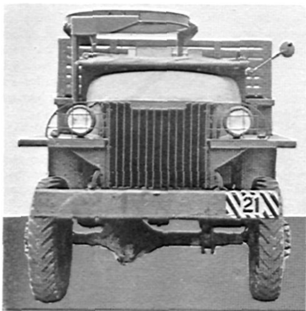
Fig. 1.—Open cab, front view. With the top down the driver's visibility is unlimited. The gun ring is low enough to preserve the "low silhouette."
