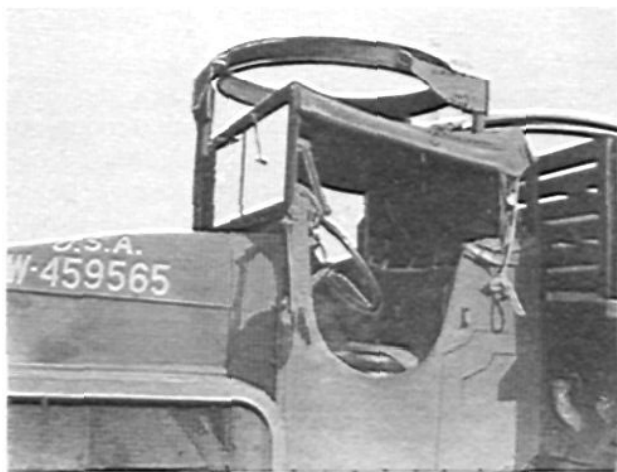
Fig. 2.—Another of the open cabs. The collapsible top and side-curtains (not in picture) shelter the driver. That's a mount for a machine gun above the top.
