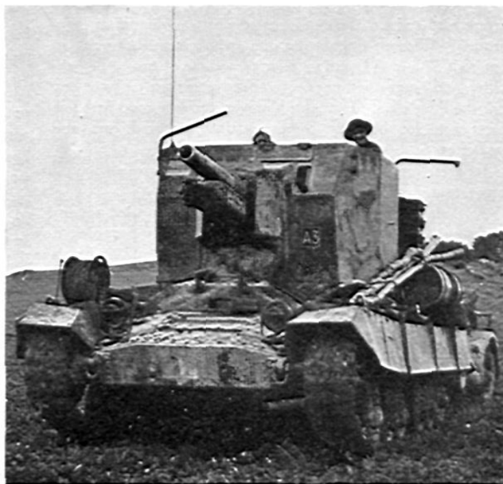
Britain's versatile 25-pdr. is now found mounted on the Valentine tank. This provides a fleet, mobile weapon, although our M7 probably has the advantage. The piece shown here is with the British First Army in northern Tunisia.
