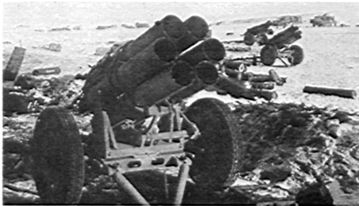
Germany's 6-barreled rocket projector is apparently mounted on a modification of the carriage used with her old 37-mm antitank guns. Ammunition packing case indicates that projectiles are about as long as the barrels.
